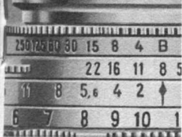
When set on B, the shutter will remain open for time exposures as long as the release is held down. It is easy to calculate a time exposure with the *green* numbers 4 to 250, indicating full seconds.
