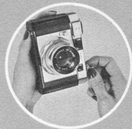
**4** The exposure counter shows how many pictures are remaining on the film. *It must be set before the back cover is replaced.* For 20 exposure roll of film, move setting dial (just above film track) with your fingertip until counter shows red 22. With a 36 exposure film, turn until counter shows red 2.
