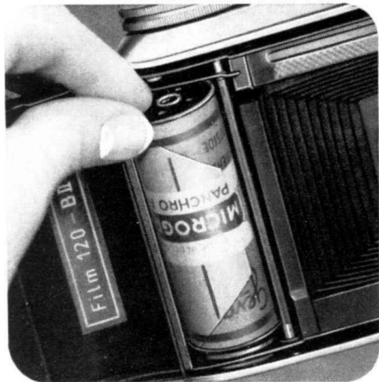
Of the two spool chambers, the one under the film winding knob holds the empty take-up spool. If it is in the other chamber, remove it and change it over (see bottom of page 14).
