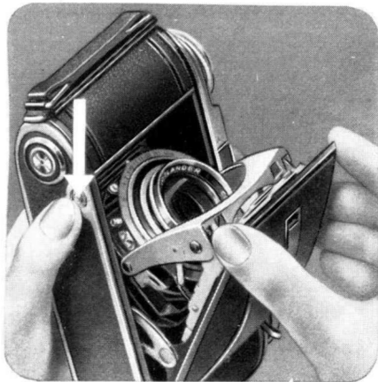
Press the small button underneath the camera to open it. Pull down the baseboard by its two corners until the struts click into position. It is then ready for use.
