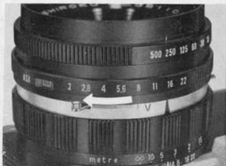
With the MX setting lever at position X, move selftimer lever (V) to cock selftimer mechanism. Operation of the shutter button will now release selftimer so that shutter action occurs about 10 seconds later.
