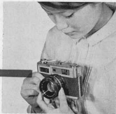
■ When presetting aperture for obtaining desired depth of field set aperture at suitable size, then turn shutter-speed ring for zero-in of exposure meter needle. Shutter-speed ring must be set at click stop, intermediate positions cannot be used. Bring needle, by click stop settings, to as close to fixed mark as possible, and make fine adjustment by aperture ring.
