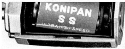
FIGURE 5. Cartridge Fits in Slot, Bottom
